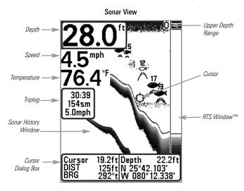
**NOTE:** If the Depth number is flashing, it means that the unit is having trouble locating the bottom. This usually happens if the water is too deep, the transducer is out of the water, the boat is moving too fast, or for any other reason that the unit can't accurately receive continuous data.
